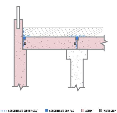
**STEP 1:** Clean joint thoroughly. Apply Xypex Concentrate slurry to joint surface at the rate of 2.0 lb./sq.yd. (1.0 kg/m²).
