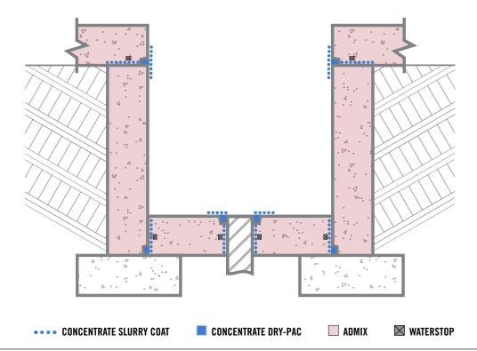
STEP 1: Where the slab will contact the wall modify the wall forms to create a linear groove in the finished concrete surface. The linear groove is to be aligned with the bottom of the slab and is to be 1½" (37 mm) high by 1" (25 mm) deep.
