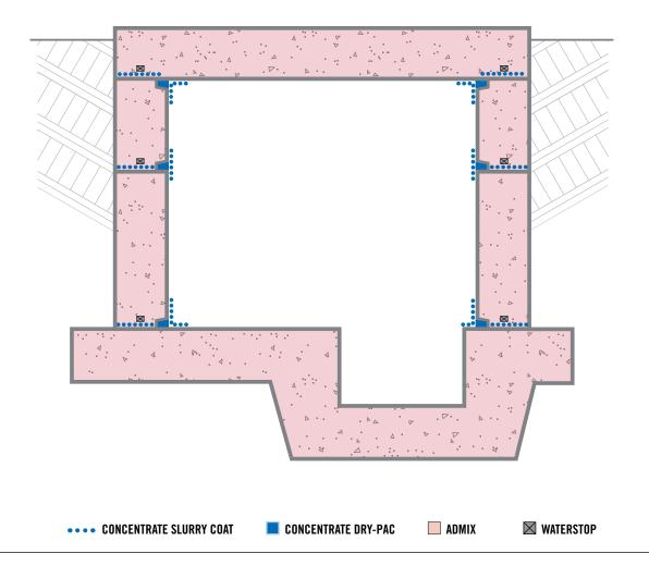
**STEP 1:** Clean joint thoroughly. Between pours apply Xypex Concentrate slurry to joint surface at the rate of 2.0 lb./sq.yd. (1.0 kg/m²).
